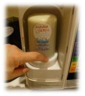
• Always check the O-ring and place back on HG filter
